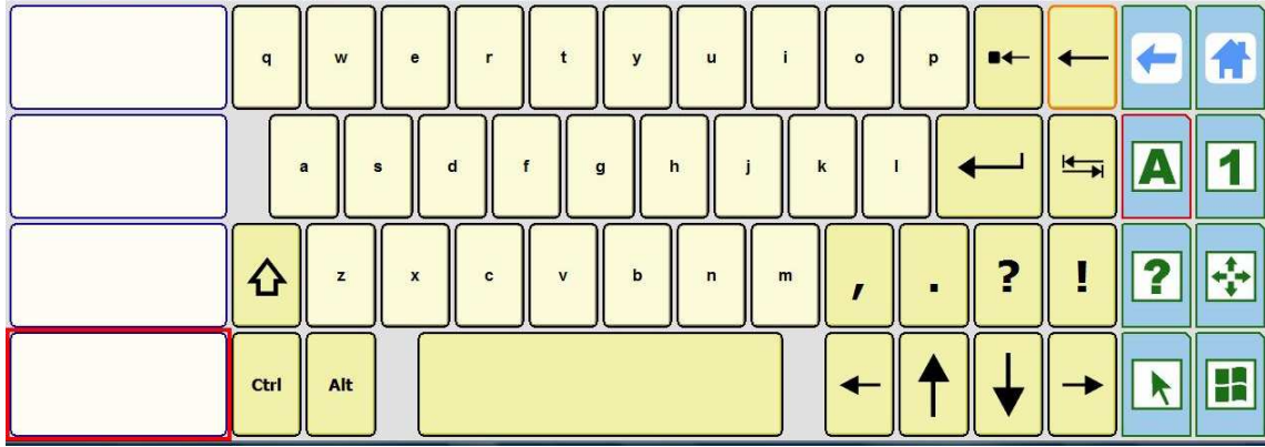
Figure 1: One of the pre-packaged scanning grids for writing in The Grid 2 commercial software (Sensory Software International Ltd., 2008). The four blank cells on the far left are designed to hold word completions, which dynamically adjust according to what has been written. The characters and functions in the remaining cells are fixed.
