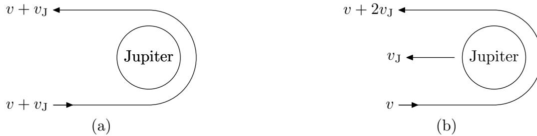
Figure 2. Bouncing off Jupiter. In the lab frame, a spacecraft approaches Jupiter with speed v , as shown in (a). Meanwhile Jupiter is doing its usual orbital motion, giving it speed v_J in the opposite direction. In Jupiter's frame, shown in (b), the spacecraft approaches with speed v + v_J , so it bounces off with the same speed. Transforming back to the lab frame shows that the spacecraft leaves Jupiter with speed v + 2v_J .
