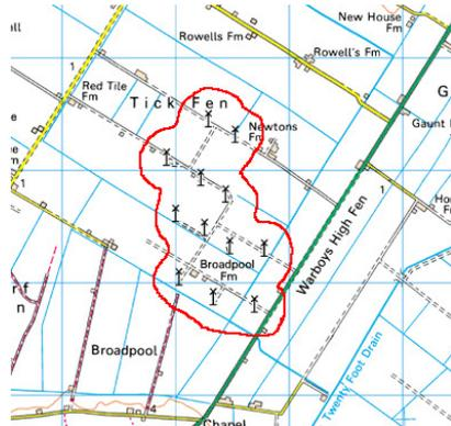
Figure 1.2. Red Tile wind farm, East Anglia, and its associated land area. The blue grid’s spacing is 1 km. Each turbine has a diameter of 82 m and a capacity of 2 MW. Map © Crown copyright; Ordnance Survey.
