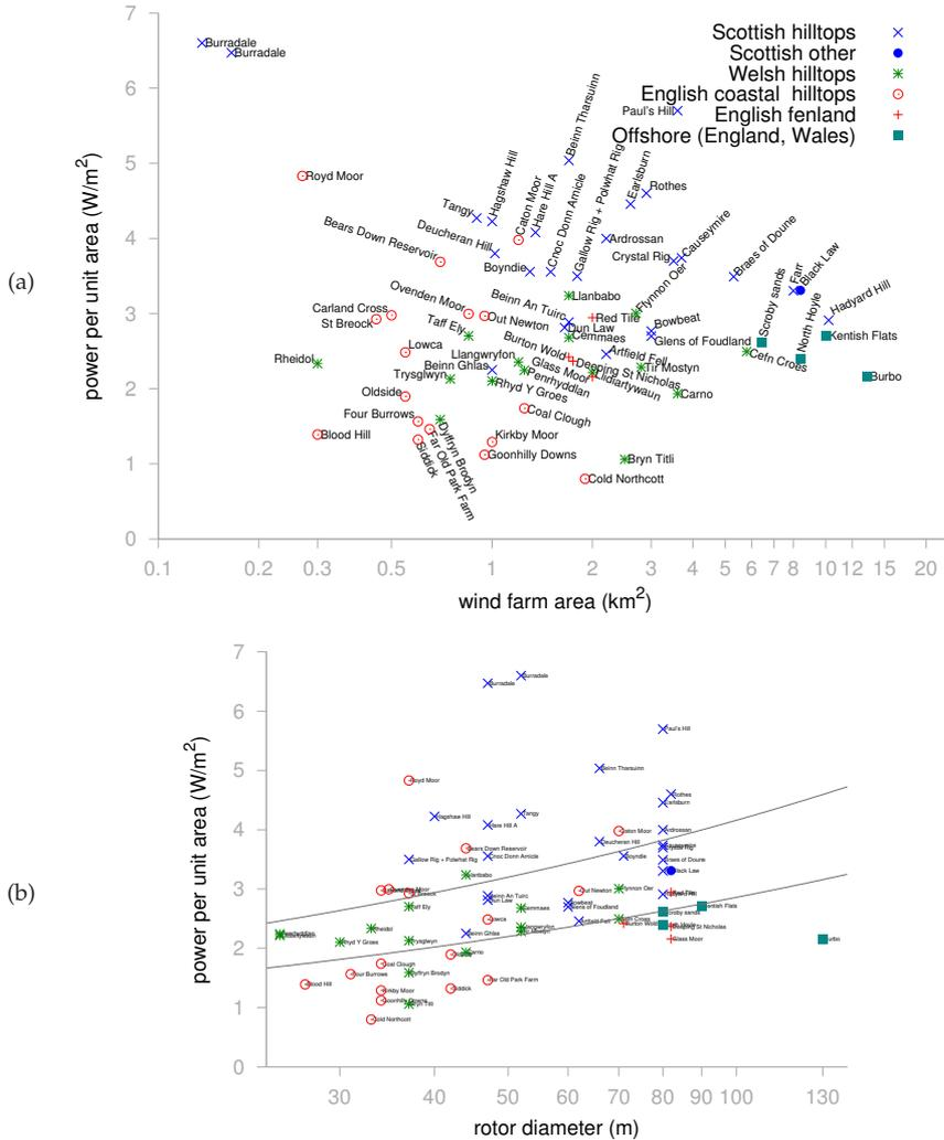
Figure 1.4. (a) Power per unit area of UK windfarms versus their size. The horizontal scale is logarithmic. (b) Power per unit area versus turbine diameter. The horizontal scale is logarithmic. The black curves in (b) show the trend that would be expected (within any single region) on the basis of the rule of thumb “doubling turbine size increases wind-speed by 10% and increases power by 30%”, and assuming wind turbines’ spacings are proportional to their diameters. From MacKay (2013).
