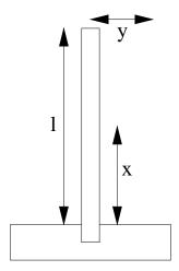
The bending moment at x due to a force at the end of the ruler is
