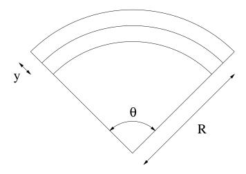
Since the length of the rod is  $l = R\theta$ , the strain in the material at y is
