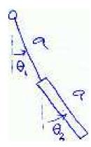
The linear velocity of the c.g. is the vector sum of the two swinging motions, but since the angle is so small they are almost parallel and so just adds:
