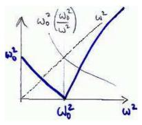
The behaviour is a bifucation at  $\omega = \omega_0$ , as shown below in the state space diagram:
