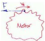
Work rate on motor =  $-Fv_1$  (i.e. motor is losing energy)
