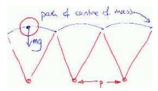
Walking involvies pivoting like an inverted pendulum. If an inverted pendulum moves fast enough then the reaction force from ground drops to zero; any faster, you'll be flying.
