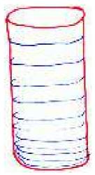
For a cylindrical rod, if we assume that it is all accelerating upwards then the strain must increase linearly towards the bottom, since we need a bigger stress to accelerate the whole mass.
