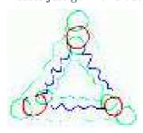
There are two degenerate (i.e. same frequency, and related by symmetry) modes corresponding to much the same two modes in (a), in which the triangle changes from being fat-short to narrow-tall. You would have thought there are three; but in fact the 3rd one is a linear combination of the other two.
