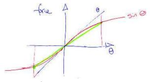
$$\begin{split} \sin\theta &= \theta - \frac{\theta^3}{6} + \ldots, \\ \text{force} &\approx \frac{\theta}{\theta_{\text{typical}}} \left\{ \theta_{\text{typical}} - \frac{\theta_{\text{typical}}^3}{6} + \ldots \right\}, \end{split}$$
