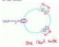
Note that even though there is a 3-fold symmetry, there are only two (degenerate) modes of this form, as the 3rd is just a linear combination (addtion, actually) of the two.
