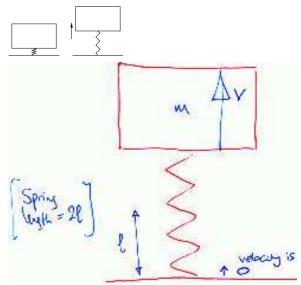
At the moment when spring stops pressing on m, its top end is going at v, like m, and its bottom end is going at 0. The spring is uniform, so its centre of mass is going at v/2.
