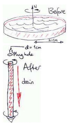
$\omega = \frac{a^2}{b^2}\Omega$ ,  $\Omega$  the rate of rotation of the earth. Using reasonable numbers  $(a=1\mathrm{m},\,b=1\mathrm{~cm})$  the rotation rate is about 1 rotation per 10 seconds.
