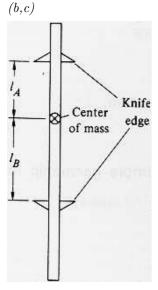
In Kater's pendulum, a pair of suspension points are found such that they have the same  $\tau^2$ , and are on different branches B and D as shown.
