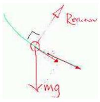
To get SHM, we need to see the equation of motion reduces to  $\ddot{s} \propto -s$ , and that means  $\frac{\partial y}{\partial s} \propto y$ . Therefore y must satisfy:  $y(s) = \frac{1}{2a}s^2$ , where a is a constant yet to be determined.
