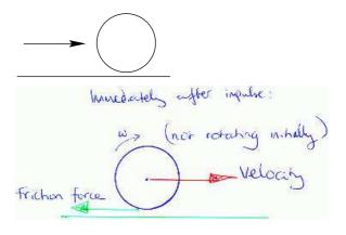
If hit along the centre, the ball would shoot forward gliding and slipping. The friction decelerates the linear motion, while making it rotate. So it rotates faster and faster, while gliding along slower and slower. At some point later, when the linear velocity has slowed down enough and the rotation has speeded up enough such that they are compatible, the ball would <u>roll</u> instead of glide/slip.
