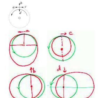
Period  $\propto a^{3/2}$ . It is possible to prove for  $V=-\frac{A}{r}$  and  $F=-\frac{A}{r^2}$  that the semi-major axis  $a=-\frac{A}{2E}\propto |E|^{-1}$  (remember E is negative, so when E increases, |E| decreases in magnitude), and the semi-lactus-rectum  $r_0=\frac{J^2}{Am}\propto J^2$ .
